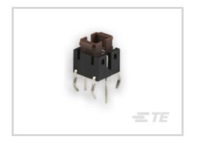
Actuator Style: Rectangular Operating Function: Off (On) Contact Base Material: Brass Switch Contact Plating Material: Silver Dust Proof: No
