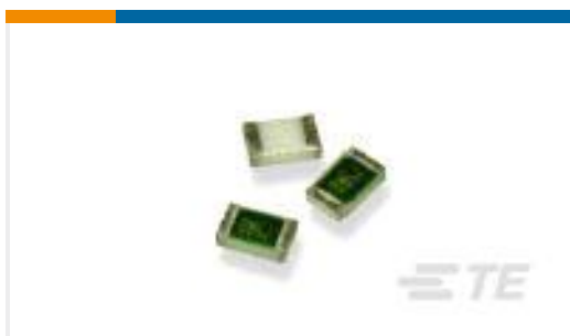
TE Part #1879417-4 CPF0603 680K 0.1% 25PPM 5K RL
