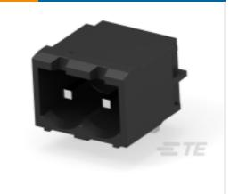
TE Part #2342079-2 2POS HDR 90 DEG,HT,5.00MM PITCH, TL 2.6MM
