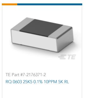
1.05K  $\Omega$ , Thin Film, Precision Resistor, .1 %, 2 Termination, 0603, Taped & Reeled, . 166 W, ±25 ppm/°C, Solder, 1.55 x .8 x .45 mm, Holsworthy RP73
