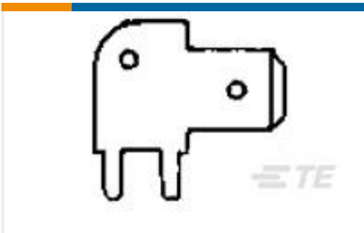
TE Part #726387-2 250 FASTON TAB TPBR
