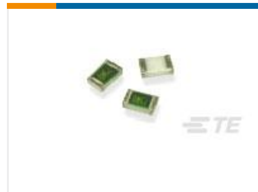
TE Part #2176087-4 RP 1J 0.166W 73R2 0.1% 25PPM 1K RL
