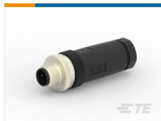
TE Part #T4111002021-000 M12,MALE,STRAIGHT,A CODE,2P, PG9,GOLD
