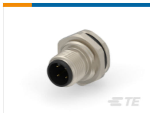
TE Part #T4171010004-001 M12,REAR MOUNTING,MALE,A,4P,0.2 M WIRE
