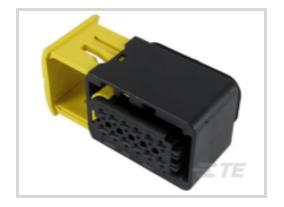
Connector System: Wire-to-Wire Number of Positions: 12 Connector & Housing Type: Housing for Female Terminals Centerline (Pitch): 4 mm [.157 in ] Sealable: Yes All Heavy Duty Sealed Connector Series Housings (204)
