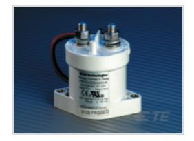
Contact Voltage Rating: 12–900 VDC High Voltage Relay Contact Arrangement: 1 Form X, SPST-NO High Voltage Connection (Coil): Flying Leads High Voltage Connection (Power): Stud Terminals Economizer: External
