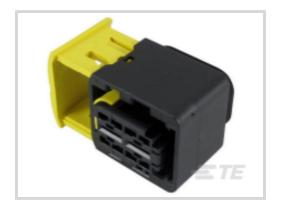
Connector System: Wire-to-Wire Number of Positions: 2 Connector & Housing Type: Housing for Female Terminals Centerline (Pitch): 9 mm [.354 in ] Sealable: Yes
