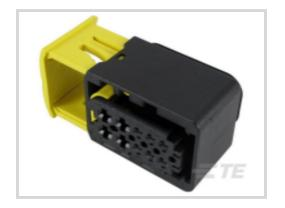
Connector System: Wire-to-Wire Number of Positions: 10 Connector & Housing Type: Housing for Female Terminals Centerline (Pitch): 4 mm, 6 mm [.157 in, .236 in ] Sealable: Yes All Heavy Duty Sealed Connector Series Housings (204)
