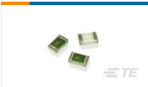
TE Part #7-2176092-0 RP 2A 0.25W 4K02 0.1% 25PPM 1K RL
