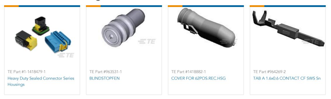
Housing for Female Terminals, Wire-to-Wire, 3 Position, .157 in [4 mm] Centerline, Sealable, Black, Signal, Heavy Duty Sealed Connector Series
