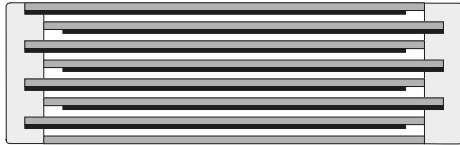
Extended metallized film design
