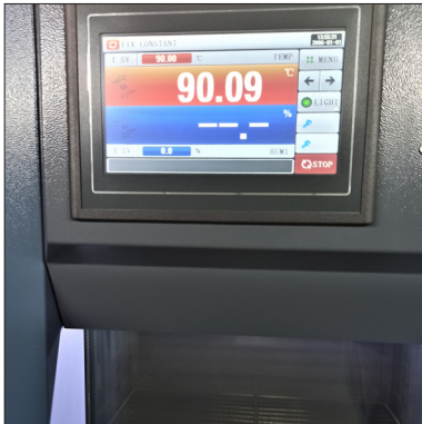
Temperature set in the climatic chamber
