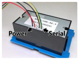
Connect the power and serial cables from the DC jack and Cobbler, noting the labels on the bottom of the printer. The connectors are identical and it's easy to get these switched around.
