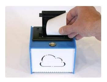
Pull up the top lever to access the paper compartment. Insert a roll of thermal receipt paper and push the lid closed while feeding the end of the paper through the slot.
