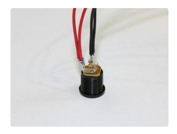
Repeat with the two black wires through the "outer" small leg (–).
