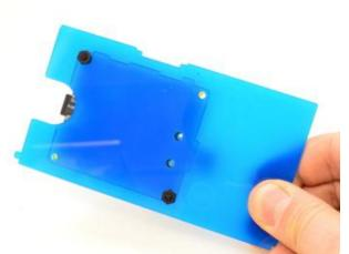
Push out the laser cut holes and mount the Raspberry Pi Board to the bottom plate using the included plastic #4-40 screws
