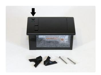
The parts baggie included with the thermal printer contains two triangle-shaped brackets and two long screws. These will hold the printer inside the case.
