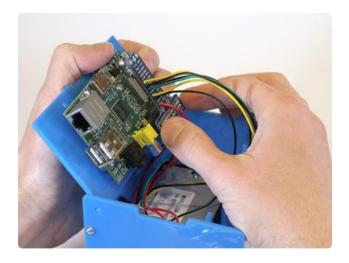
For the pre-2017 kit: Gently install the Cobbler board on to the Raspberry Pi GPIO header. Support the Pi board from below with the tips of your fingers...this prevents strain on the board and the case.
