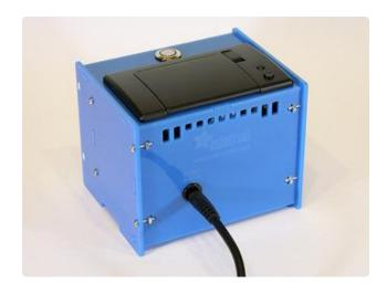
Connect the 5V DC power supply to the jack on the back of the case.
