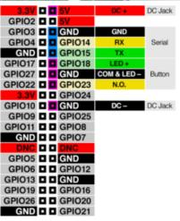
For the 2017-and-later kit, plug in the connections as shown here.
