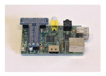
After soldering (and allowing some time to cool), you can test fit the Cobbler on the Raspberry Pi. Gently pry it off with your fingers afterward...more soldering lies ahead...
