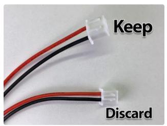
Cut the red/black power cable in half. This cable has a different plug at each end. We want to keep the wider of the two plugs for the printer; the other can be discarded or tossed in your spare bits drawer.
