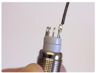
Loop the BLACK wire through the LED – and COMMON pins, bend it back on itself and solder.
