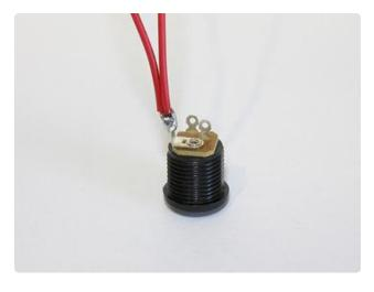
Twist the two red wires together, feed through the large center leg (+) and solder in place.
