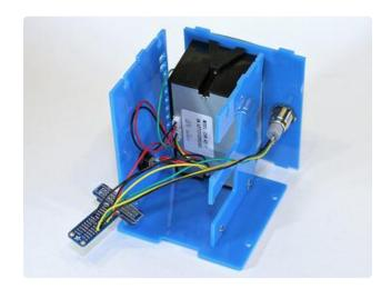
Stand the partial case up on its side and move the top piece (with button and thermal printer attached) roughly into position. Don't fit this into the slots yet, just an approximate position.
