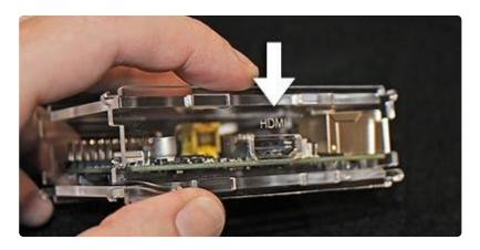
10. Install the first end of the case: slide the top of the end piece over the two top hooks first, then, using very light pressure, pivot the end piece downward over the bottom two hooks. It should click into place without difficulty. If you encounter ANY resistance, stop! Do not force this piece or you will break the plastic. Back off, check the alignment of the other pieces (especially the HDMI side), and try again. Gently. And remember, top to bottom — the other direction will break.
