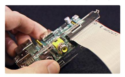
6. On the underside of the board, under the Ethernet jack, install the small spacer piece that was snapped out in Step 2.
