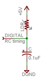
In this case, our 'bucket' is a 0.1uF ceramic capacitor. You can change the capacitor nearly any way you want but the timing values will also change. 0.1uF seems to be an OK place to start for these photocells. If you want to measure brighter ranges, use a 1uF capacitor. If you want to measure darker ranges, go down to 0.01uF.
