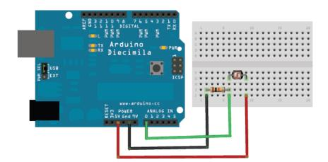
For this example I'm showing it with a 5V supply but note that you can use this with a 3.3v supply just as easily. In this configuration the analog voltage reading ranges from 0V (ground) to about 5V (or about the same as the power supply voltage).
