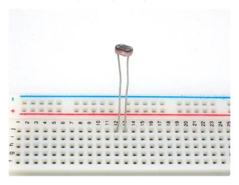
Photocells are pretty hardy, you can easily solder to them, clip the leads, plug them into breadboards, use alligator clips, etc. The only care you should take is to avoid bending the leads right at the epoxied sensor, as they could break off if flexed too often.
