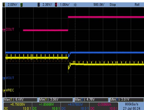
Figure 13. Load Transient: V_{OUT} = 4.5V , 0A \rightarrow 1.2A
