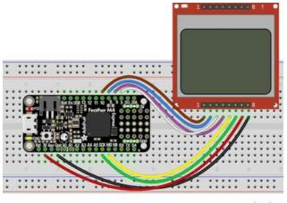
Microcontroller GND to LCD Gnd
