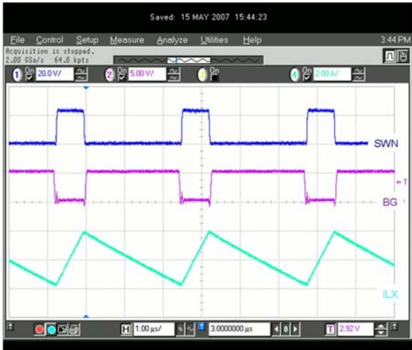
Figure 22. Switcher Operation – CCM Mode
