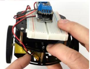
The AA batteries will supply power to the motors through the Motor Driver FeatherWing, but what about power for the Feather itself? For that, you'll use a LiPoly battery. It's small, powerful, and very convenient -- you can charge it simply by plugging the Feather into a USB charger!
