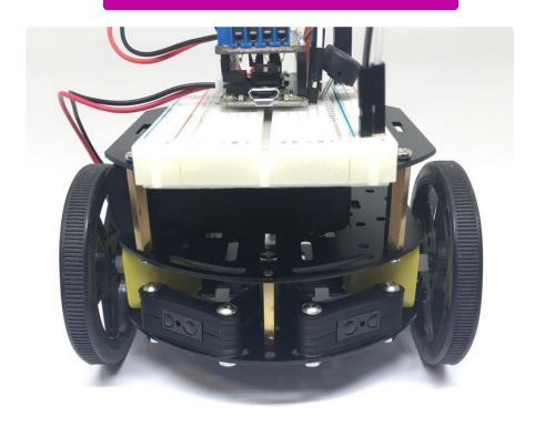
I used a couple M2.5 screws to secure the mounts to the robot (required a drill bit to clean up the holes in the 3D print). I wired up the left sensor to pin A4, and the right sensor to pin A5.
