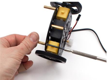
Take a look at the image below and install the brass stand-offs in the same positions. You can insert the stand-off screws through the middle plate and hand tighten the stand-offs while putting a bit of pressure on the screw with your finger. Or, as a tip, you can screw in the stand-off screws with the flat end of the screwdriver, which can reach through the holes in the bottom plate.
