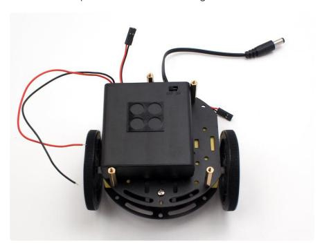
Notice the battery box is lined up on the left side of the middle chassis plate. It should be just in-between the upper left stand-off and the lower left stand-off (not touching either). This will make sure the on-off switch lines up just right in the hole of the top plate. Go ahead and install the top plate now as shown here.
