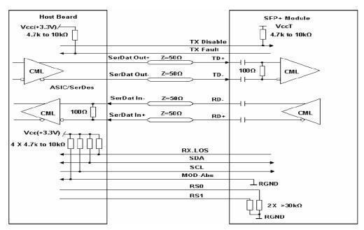
**Recommended High-speed Interface Circuit**
