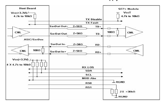
**Recommended High-speed Interface Circuit**
