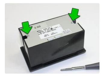
Unplug all cables, turn the printer over and remove the two small Phillips screws.
