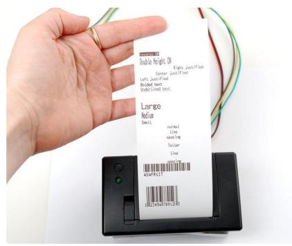
The thermal printer has a few handy things it can do, most of which are in the A\_print ertest sketch. These are shown in the image above. In order, starting from the top:
