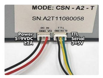
The Mini thermal printer has two 3-pin sockets—one for power, one for serial communication. Power goes to the jack labeled "DC IN." Only the outer two pins of this connector are used.
