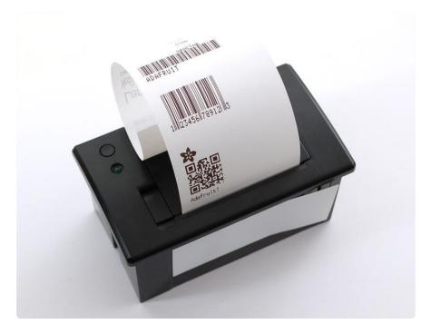
Add printing to any microcontroller project with these very cute thermal printers. Also known as receipt printers, they're what you see at the ATM or grocery store. Now you can embed a little printer of your own into a project. These printers is ideal for interfacing with a microcontroller, you simply need a 3.3V to 5V TTL serial output from your microcontroller to print text, barcodes, bitmap graphics, even a QR code!
