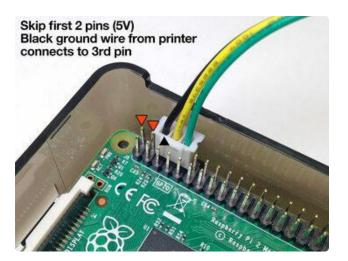
If you happen to be using the Mini printer with the 3-pin data cable, and if the Pi and printer are kept close together, you might not even need jumper wires. Skip the first two 5V pins on the GPIO header, and the data cable can press right on to the next 3 pins in sequence: GND, TX and RX.
