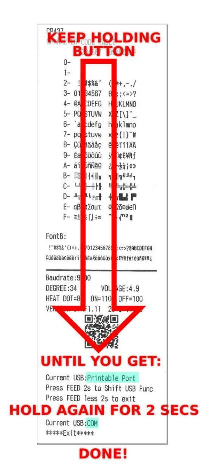
This is present only in older Tiny printers. Current units work strictly in USB printing subsystem mode—it's considered more modern—and continuing to hold the paper feed button will just eject a lot of paper...so don't.
