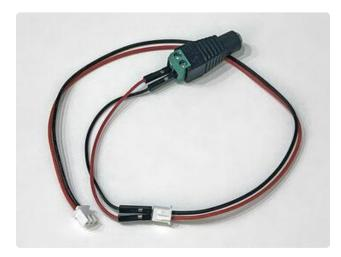
During initial testing and for quick temporary projects, it's usually okay to jam breadboard prototyping wires () into the end connector on the DC power cable (or power+serial cable on Nano and guts), and the other end to a DC barrel jack adapter.
