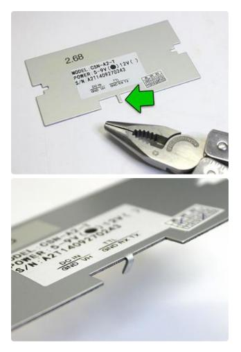
On the back plate, there's a small metal "finger" between the serial and power sockets. Using pliers, this can be bent back to provide an exit route for the DTR wire.
