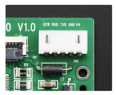
The pin order here is not the same as the Tiny or Nano printers. And if you have both Guts and Nano printers, be super careful about the wiring, because the plugs are
