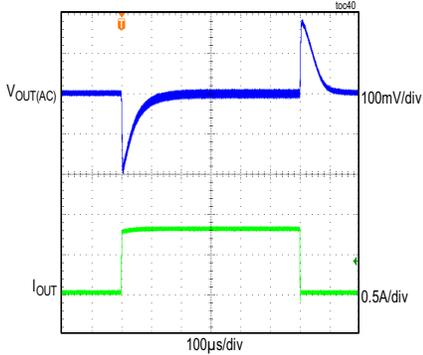
CONDITIONS: FIXED 5V OUTPUT, DCM MODE,  $f_{SW} = 400kHz$
