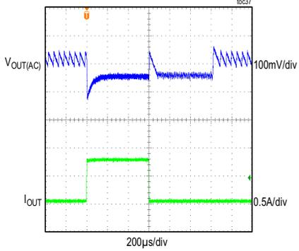
CONDITIONS: FIXED 3.3V OUTPUT, PFM MODE,  $f_{SW} = 400kHz$
