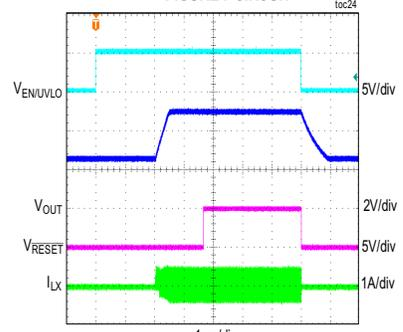
CONDITIONS: ADJUSTABLE 5V OUTPUT, PWM MODE, 20mA LOAD,  $f_{SW} = 850kHz$
