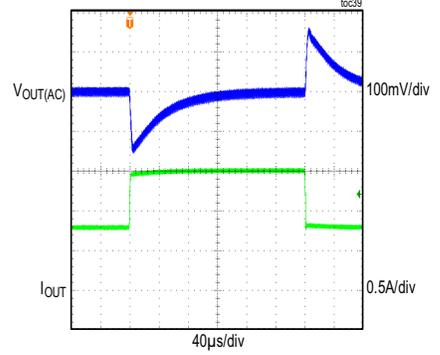
CONDITIONS: FIXED 5V OUTPUT, PWM MODE,  $f_{SW} = 400kHz$
