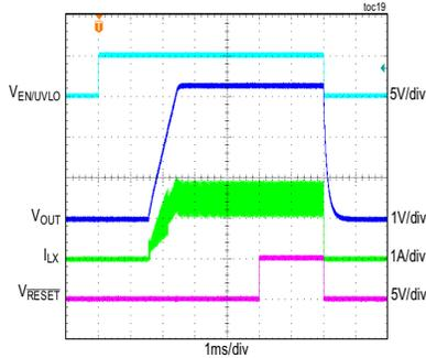
CONDITIONS: FIXED 3.3V OUTPUT, PWM MODE, 1.5A LOAD,  $f_{SW} = 400kHz$
