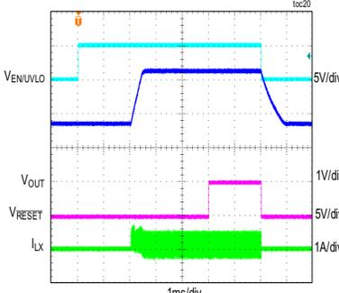
CONDITIONS: FIXED 3.3V OUTPUT, PWM MODE, 20mA LOAD,  $f_{SW} = 400kHz$
