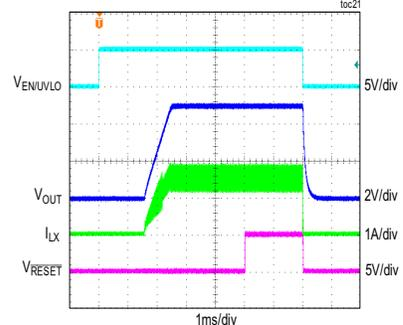
CONDITIONS: FIXED 5V OUTPUT, PWM MODE, 1.5A LOAD,  $f_{SW} = 400kHz$
