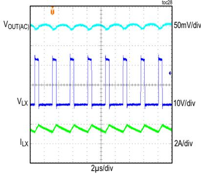
CONDITIONS: FIXED 5V OUTPUT, PWM MODE, 1.5A LOAD,  $f_{SW} = 400kHz$
