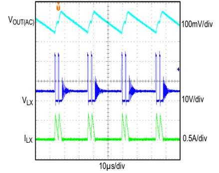
CONDITIONS: FIXED 5V OUTPUT, PFM MODE, 20mA LOAD,  $f_{SW} = 400kHz$
