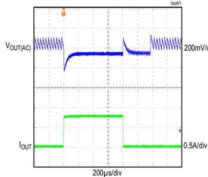
CONDITIONS: FIXED 5V OUTPUT, PFM MODE,  $f_{SW} = 400kHz$
