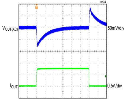
CONDITIONS: FIXED 3.3V OUTPUT, PWM MODE,  $f_{SW} = 400kHz$
