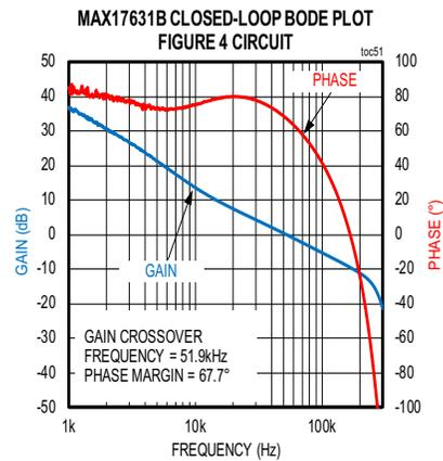
CONDITIONS: FIXED 5V OUTPUT, PWM MODE, 1.5A LOAD,  $f_{SW} = 400kHz$
