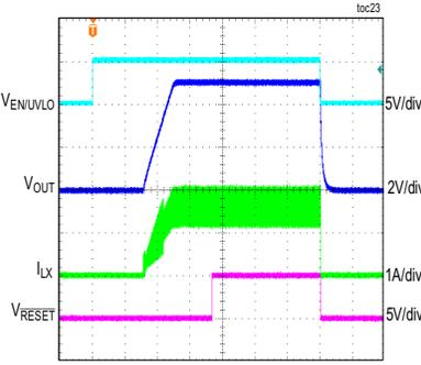
CONDITIONS: ADJUSTABLE 5V OUTPUT, PWM MODE, 1.5A LOAD,  $f_{SW} = 850kHz$
