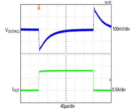
CONDITIONS: ADJUSTABLE 5V OUTPUT, PWM MODE,  $f_{SW} = 850kHz$
