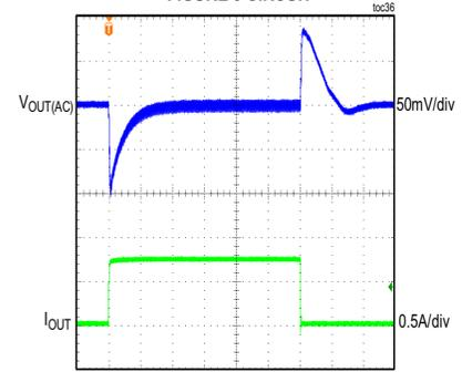
CONDITIONS: FIXED 3.3V OUTPUT, DCM MODE,  $f_{SW} = 400kHz$
