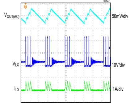
CONDITIONS: FIXED 3.3V OUTPUT, PFM MODE, 20mA LOAD,  $f_{SW} = 400kHz$
