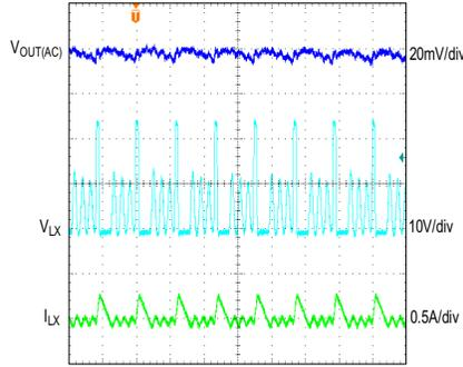
CONDITIONS: ADJUSTABLE 5V OUTPUT, DCM MODE, 40mA LOAD,  $f_{SW} = 850kHz$
