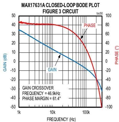
CONDITIONS: FIXED 3.3V OUTPUT, PWM MODE, 1.5A LOAD,  $f_{SW} = 400kHz$
