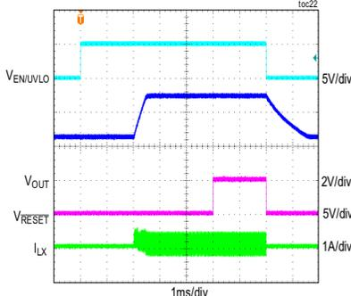
CONDITIONS: FIXED 5V OUTPUT, PWM MODE, 20mA LOAD,  $f_{SW} = 400kHz$
