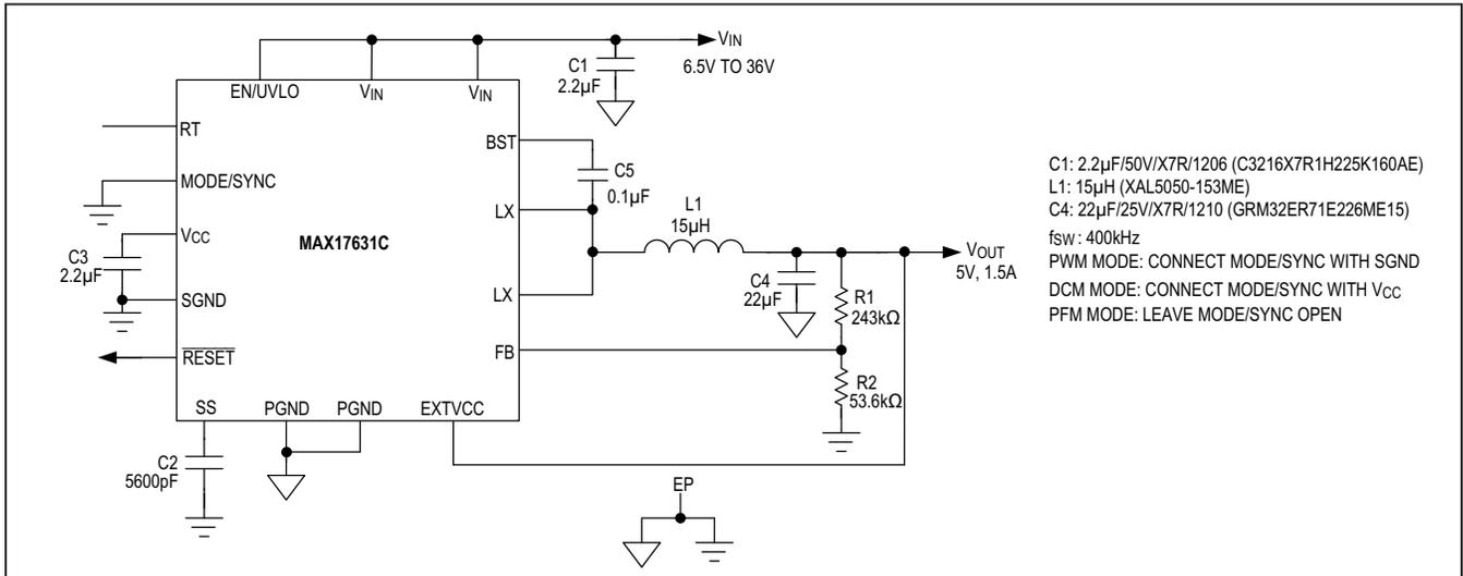
Figure 6. Adjustable 5V Output with 400kHz Switching Frequency
