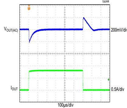
CONDITIONS: ADJUSTABLE 5V OUTPUT, DCM MODE,  $f_{SW} = 850kHz$
