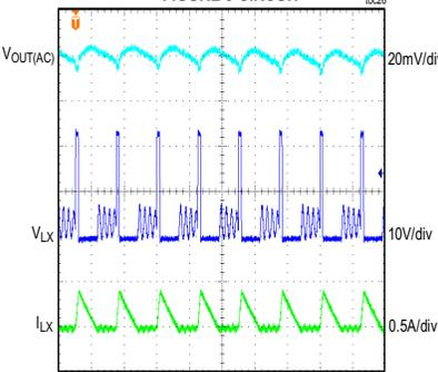
CONDITIONS: FIXED 3.3V OUTPUT, DCM MODE, 40mA LOAD,  $f_{SW} = 400kHz$
