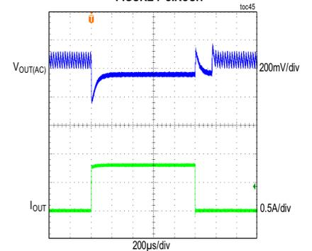
CONDITIONS: ADJUSTABLE 5V OUTPUT, PFM MODE,  $f_{SW} = 850kHz$
