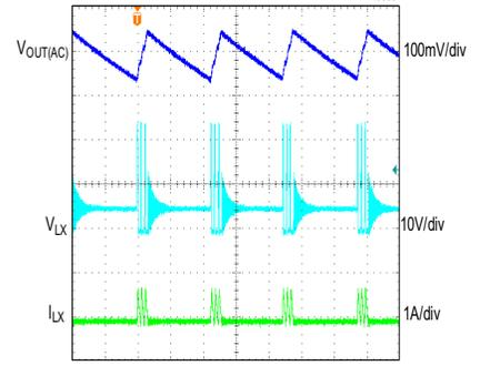
CONDITIONS: ADJUSTABLE 5V OUTPUT, PFM MODE, 20mA LOAD,  $f_{SW} = 850kHz$
