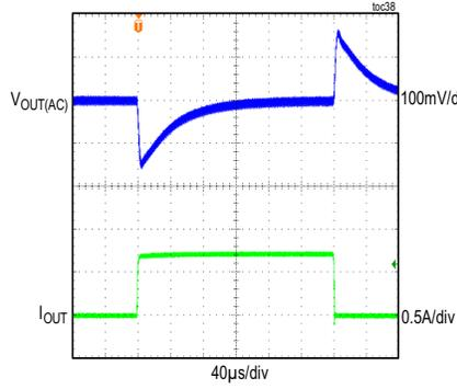
CONDITIONS: FIXED 5V OUTPUT, PWM MODE,  $f_{SW} = 400kHz$
