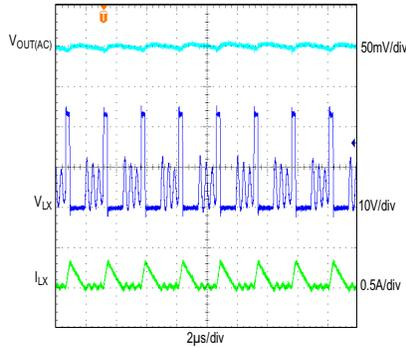
CONDITIONS: FIXED 5V OUTPUT, DCM MODE, 40mA LOAD,  $f_{SW} = 400kHz$
