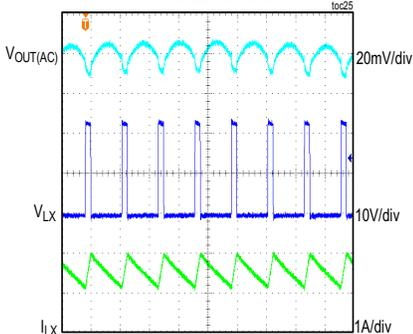
CONDITIONS: FIXED 3.3V OUTPUT, PWM MODE, 1.5A LOAD,  $f_{SW} = 400kHz$
