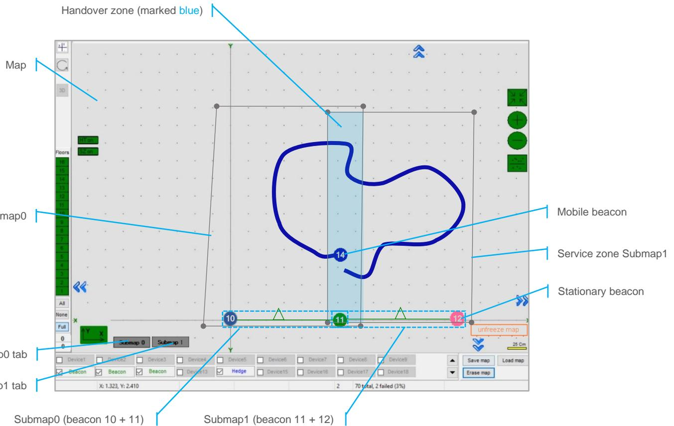
The main parameters of a submap are its **size**, **frequencies** and **TDMA (Time Division Multiple Access) position** of stationary beacons, by which mobile beacons can not only be positioned, but also determine in which submap the mobile beacon is located.
