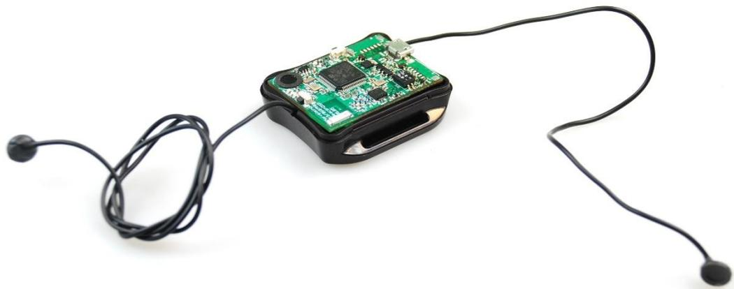
Figure 2: Two external microphones with housing
