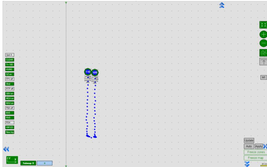
Beacons must be at least 20 cm apart. The farther the beacons are from each other, the more accurate the angle. Also, if beacons are so close to each other it's better to connect it via UART, to avoid issues with tracking.
