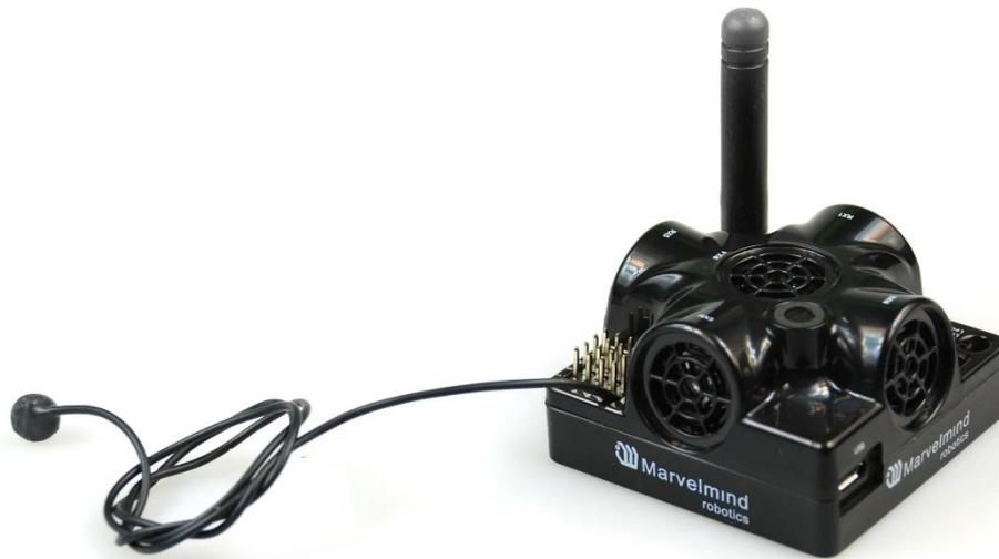
*Figure 1: Super-Beacon with one External Microphone connected*
