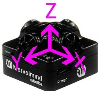
Mini-RX beacon IMU axis positions
