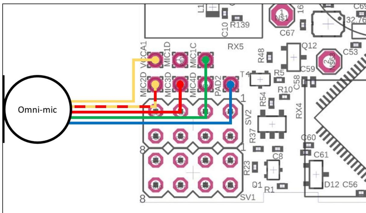
Figure 5: Omni-Microphone connection for Super-Beacon-2 and Super-Beacon-3
