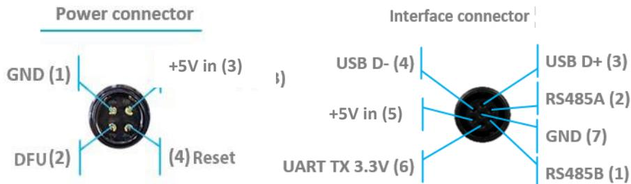
Version 2 and 3 of Industrial-TX-Metal (from June 2022) **supports ONLY +5V power supply**. Don't use +12V power supply converter for this version, it will burn the beacon!
