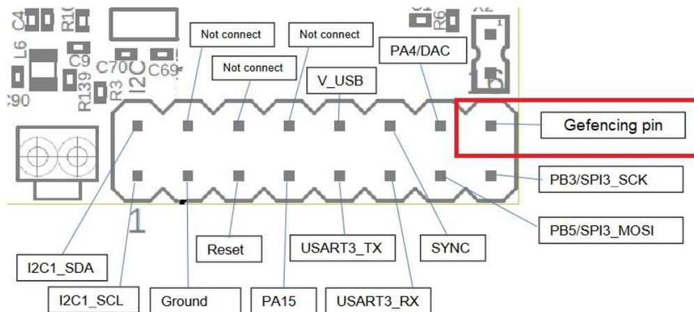
9.7.1.3. Geofencing pin scheme for Mini-RX:
