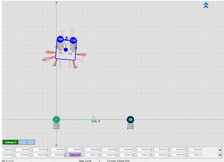
Moreover, each beacon streams out in this mode not only its own location, but direction where the pair is facing. This feature hugely simplifies autonomous driving and flight. Here is an updated [protocol](#) with the changes.
