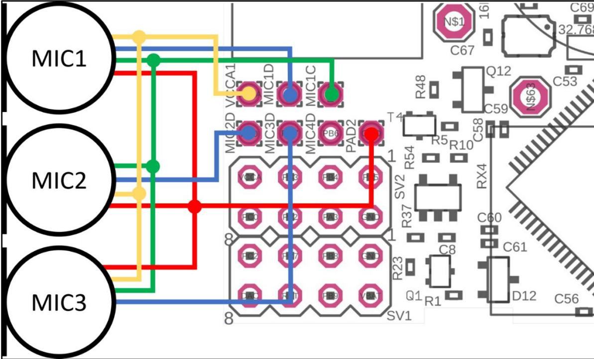
Figure 8: Two External Microphone connection
