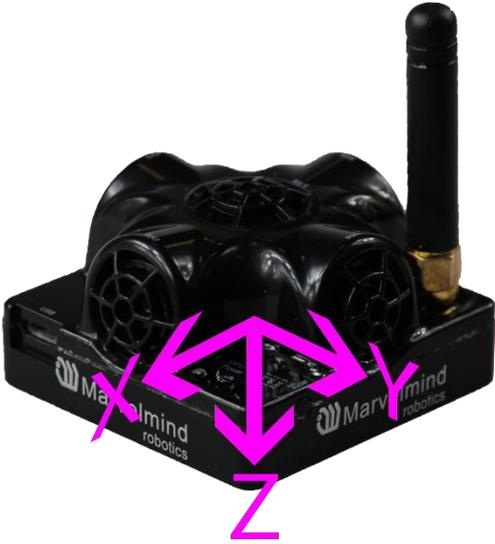
Mini-TX IMU axis positions
