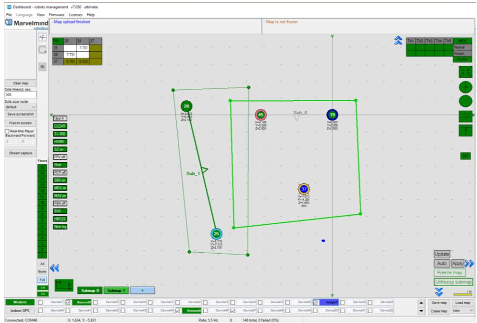
Initial height of the service zone is set up by the height of the stationary beacons. There are two layers: top and bottom. Top – the height of the stationary beacons. Bottom – by default is floor: 0 meters.
