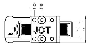
MA009253 USB Type-C Test Connector is 24-pin double sided connector with straight signaling. It is designed for testing of USB Type-C interface. The transmission of high data rates can be achieved, recommended to be verified by our customers in their applied test setup.
