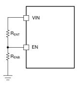
Figure 8-3. System UVLO by Enable Divider
