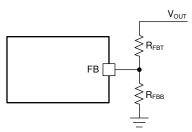
Figure 8-2. Output Voltage Setting
