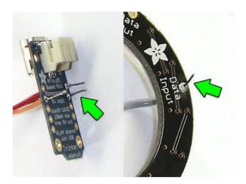
First, if you haven't already, clip off the tips of the soldered wires.
