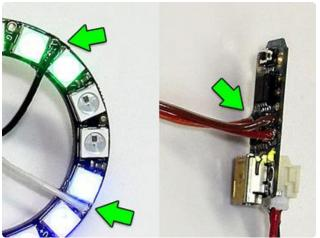
This step is optional but recommended: if you have some 5-minute epoxy or craft adhesive such as E6000, add a small bead at the base of each wire where it meets the board...and especially on the LiPoly battery and JST connector. This creates a strain relief, so wires aren't likely to break off when flexed. On the NeoPixel rings, it helps the wires sit flat.
