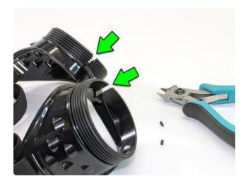
The costume goggles have slots near the nose piece, bridged by a tiny bit of plastic. If these are clipped away, then all the electronics can be slid in place from the front. You might also cut the slots just a little wider so they don't gouge the wires.
