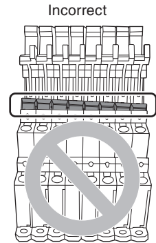
Incorrect installation Some terminals not inserted completely. Incorrect
