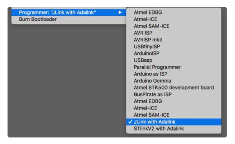
You can then click the Burn Bootloader menu entry and the Arduino IDE will attempt to use the JLink or STLink (via AdaLink ()) to reflash the bootloader for you.
