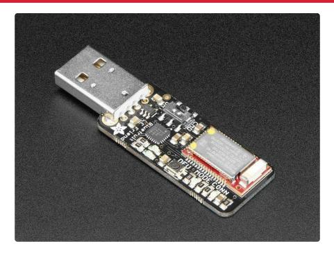
Since nRF-Sniffer is a passive solution that is simply scanning packets over the air, there is the possibility of missing packets using this tool (or any other passive sniffing solution). In order to capture as many packets as possible, be sure to run the sniffer on a USB bus that isn't busy and avoid running it in a virtual machine since this can introduce significant latency over USB.
