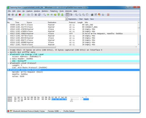
What this write request is trying to do is enable the 'notify' bit on the <u>UART service's</u>
