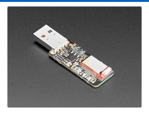
In it's simplest form, it works on the same principle as a common USB/Serial adapter (the <u>FTDI Friend</u> (), for example!). Any data that you enter via your favorite terminal emulator on your development machine will be transferred over the air to the connected phone or tablet, and vice versa.
