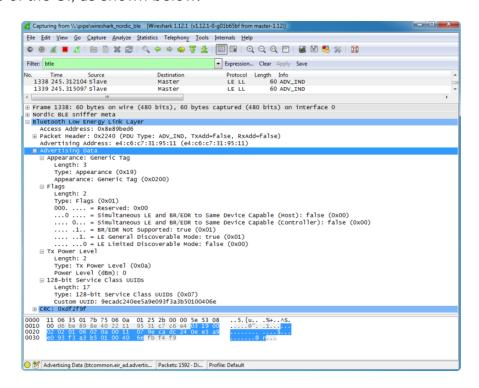
Clicking on the Advertising Data entry in the treeview will highlight the relevant section of the raw payload at the bottom of the screen, but also provides human
