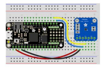
Board 3V to sensor VCC Board GND to sensor GND Board SCL to sensor SCL Board SDA to sensor SDA
