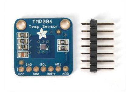
Unlike most temperature sensors, the TMP006 does not require contact with the object it is measuring. It uses a very sensitive thermopile to measure the infrared energy being emitted from the surface of the object.
