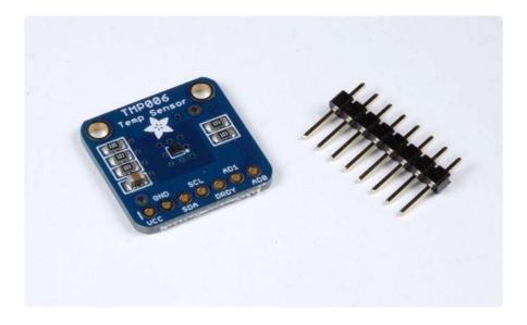
The TMP006 Thermopile Breakout comes with all surface-mount components presoldered. For use on a breadboard you will want to solder in the supplied header.
