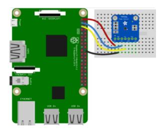
Pi 3V3 to sensor VCC Pi GND to sensor GND Pi SCL to sensor SCL Pi SDA to sensor SDA
