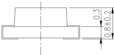
For reflow soldering (propose)
