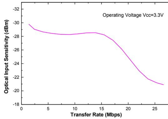
**Note:** Before using the PLR162 device, please confirm the minimum sensitivity at different operating voltage and transmission rate.
