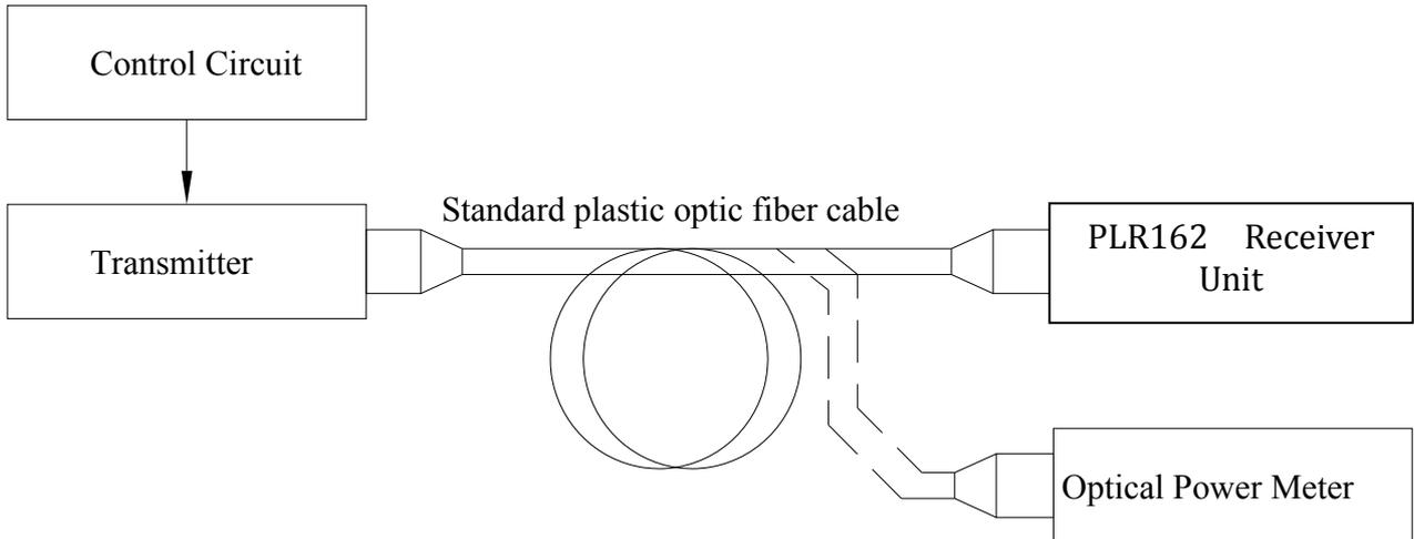
\*Fig.2 Measuring Method of Dissipation Current
