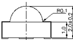
For reflow soldering (propose)
