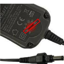
(3) Insert correct plug with GND outside
