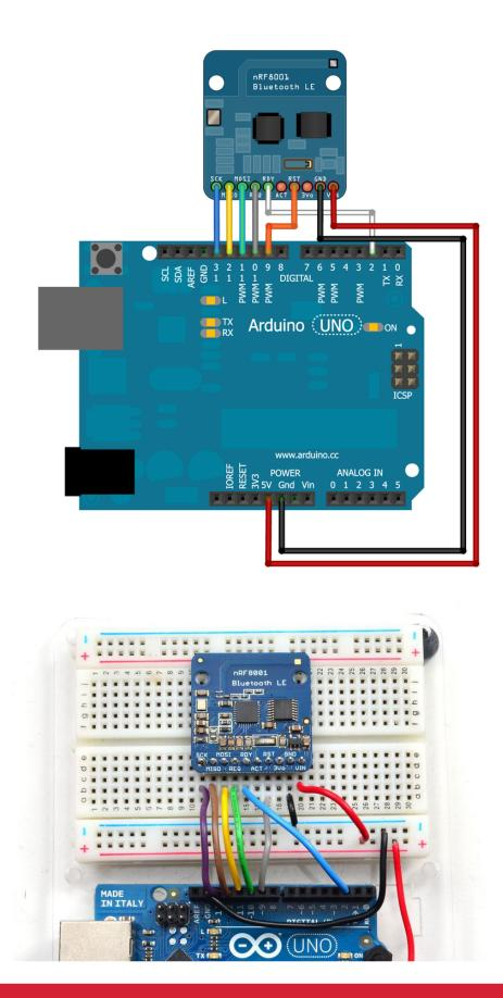
The nRF8001 differs from a classic SPI bus since CS is replaced by two pins, REQ and RDY, but you can still use HW SPI since CS is normally controlled purely in SW anyway.
