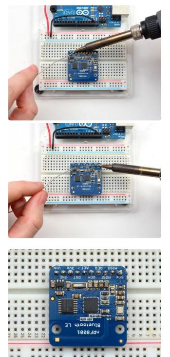
And Solder! Be sure to solder all 10 pins for reliable electrical contact.
