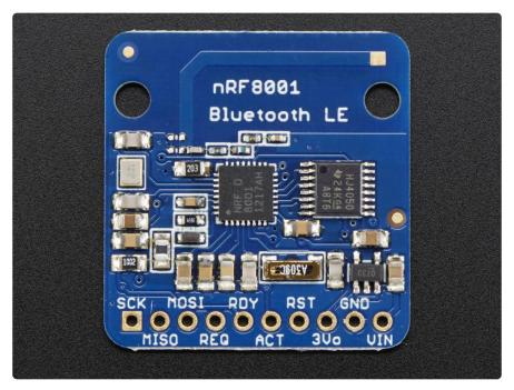
The nRF8001 is nice because it handles all the BLE radio and low level work, and does it all over SPI which makes it easy to use with any kind of microcontroller. All pins you need are broken out on the bottom of the PCB and all are 5V compliant so you can use with 3V or 5V micros!
