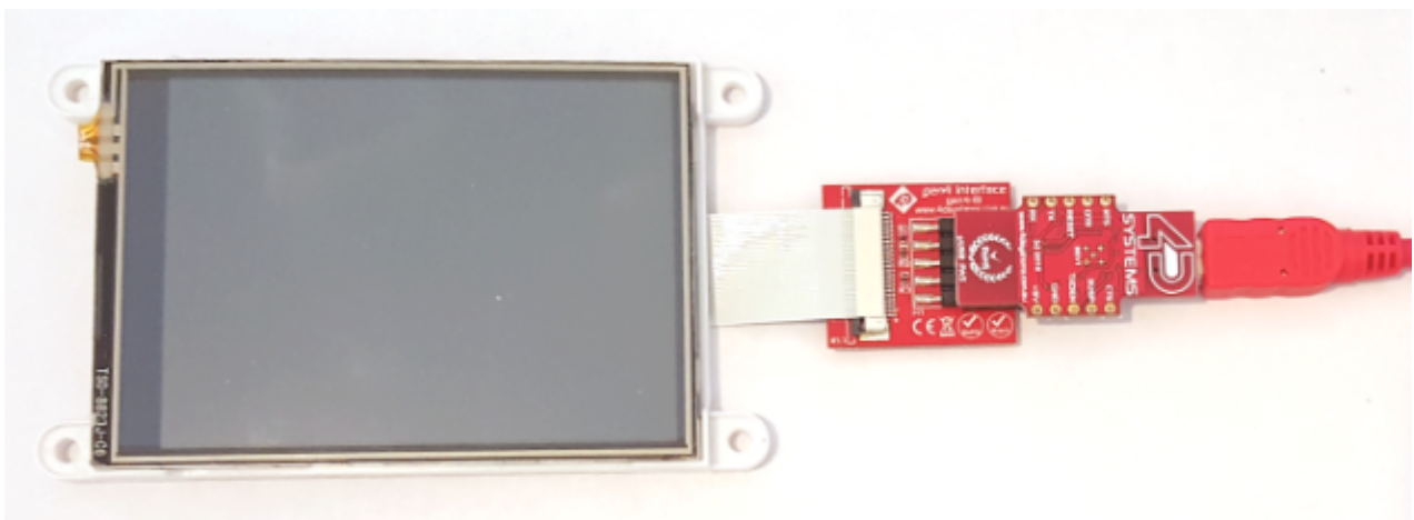
gen4 display, connected to the gen4-IB, with the uUSB-PA5 programming adaptor connected directly
