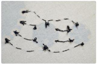
Stitching the sensor into a project is easy-just line up the sensor so its adjacent to the SDA/SCL pins on Flora or another I2C sensor, and stitch the four connections with conductive thread. This is covered in more detail in the Flora Accelerometer () guide and our Conductive Thread () guide.
