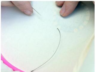
Bring your needle through the back of the fabric to the front next to the GND pad on your Flora. Leave a the last few inches as a tail on the back side of the fabric.
