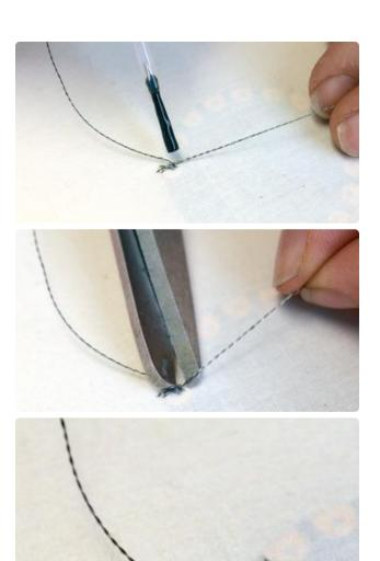
Dab a little Fray Check or clear nail polish on the knot while holding it tight. This will prevent the knot from coming undone and creating unwanted shorts in your circuit. Trim the tail very close to the knot.
