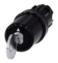
key-operated switch Siemens, 22 mm, round, plastic, lock number SSG10, with 2 keys, 3 switch positions I>O<II, momentary contact on the left, latching on the right, actuating angle  $2x45^{\circ}$ , 10:30h/12h/13:30h, key removal O+II, with laser labeling, lower case
