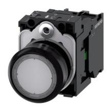
Illuminated pushbutton, 22 mm, round, plastic, clear, pushbutton, flat, momentary contact type, with holder, 1NO, LED module with integrated LED 110 V AC, screw terminal, with laser labeling, lower case
