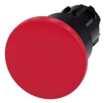
Mushroom pushbutton, 22 mm, round, plastic, red, 40mm, latching, pull-to-unlatch mechanism, with laser labeling, upper case and lower case, always upper case at the beginning of the word
