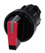
Selector switch, illuminable, 22 mm, round, plastic, red, selector switch, short, 3 switch positions I>O<II, momentary contact on the left, latching on the right, actuating angle  $2x45^{\circ}$ , 10:30h/12h/13:30h Z=50-unit packaging
