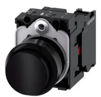
Pushbutton, 22 mm, round, plastic, black, pushbutton, raised, momentary contact type, with holder 1 NC, screw terminal, with laser labeling, upper case
