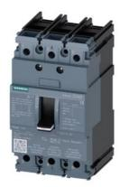
molded case switch 3VA5 UL frame 125 max. sh-circ breaking capacity 65kA @ 480 V 3-pole, line protection MCS110, In=100A without overload protection self-protection li=16 x In nut keeper kit on both sides
