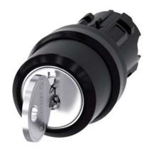
RONIS key-operated switch, 22 mm, round, plastic, lock number SB30, with 2 keys, 3 switch positions I>O<II, momentary contact on the left, latching on the right, actuating angle 2x45°, 10:30h/12h/13:30h, Key removal II, possible special locks: SB31, 421, 455, with laser labeling, inscription or symbol Customer-specific selection with SIRIUS ACT configurator (CIN)
